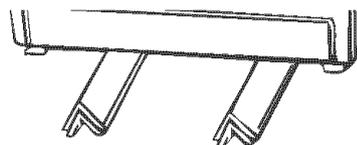
2. Use the leveling legs and nuts from parts package. Screw nut down to within 1/2" (1.3 cm) of base.
